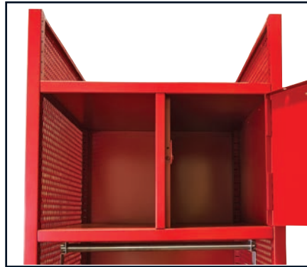
OPTIONAL SECURITY BOX USES TWO HEAVY-DUTY 13 GAUGE 7-KNUCKLE 3-1/2" HINGES AND A FINGER PULL PADLOCK HASP
