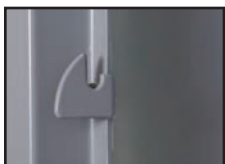
Main door latch hooks welded to frame
